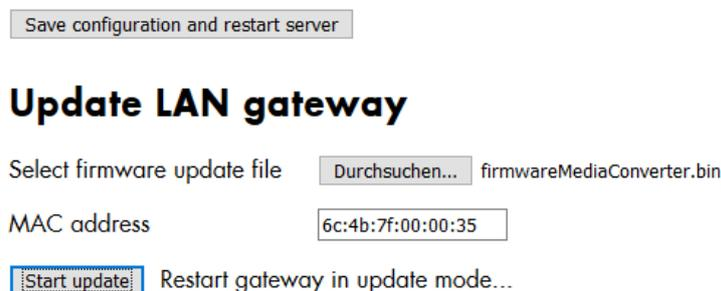
Figure 23: The Blu2Light LAN Gateway is put into "update mode"
