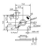
The clearance and creepage distances are designed for operation with SELV drivers. Alternativly for fixing with LED holders the Comfort COBs can be fixed with screws. Then the wires must be soldered to the solder pads.
